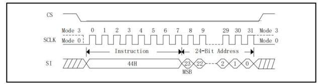
Figure 32. Erase Security Registers instruction Sequence Diagram
