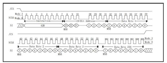
Figure 33. Program Security Registers instruction Sequence Diagram
